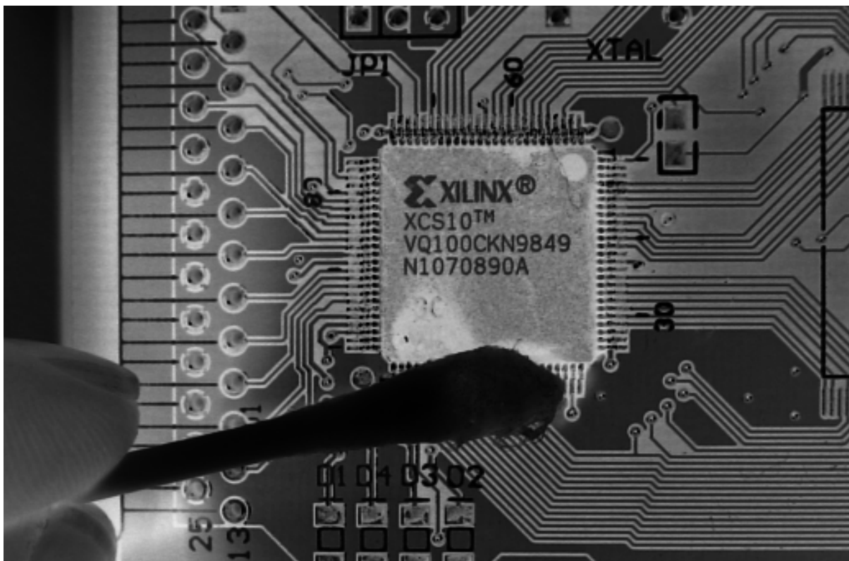
Рисунок В-5. Stroke the pins along the side of the chip using a pair of tweezers or a needle using a firm, steady force. Pins that are not soldered well will bend slightly. The arrow indicates the direction of motion.
